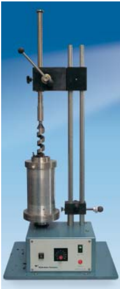
Drilling the centre hole
