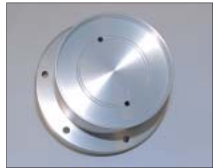
Base pedestal showing pore pressure parts without high air entry stone
