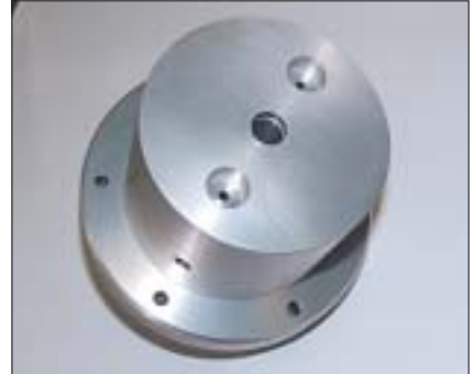
Pedestal showing the hole for suction transducer. Two access for high air entry stones
