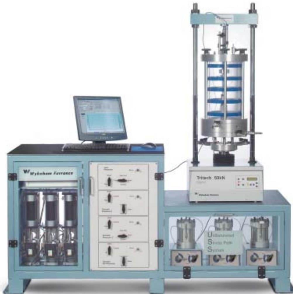
Unsaturated stress path system with provision for permeability tests. It includes 3 pressure controllers, 3 volume change and on air control valve
