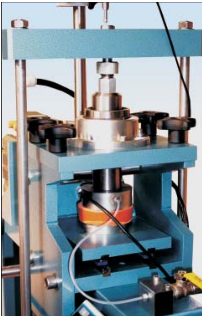
Sample having in the WF 25735 cyclic simple shear machine
