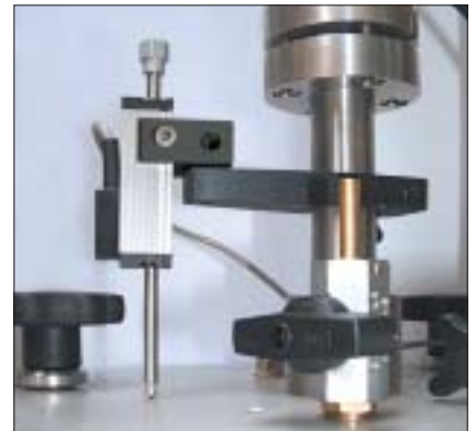
Axial displacement transducer fitted on triaxial cell with mounting bracket WF 17057 and mounting block WF 17082
