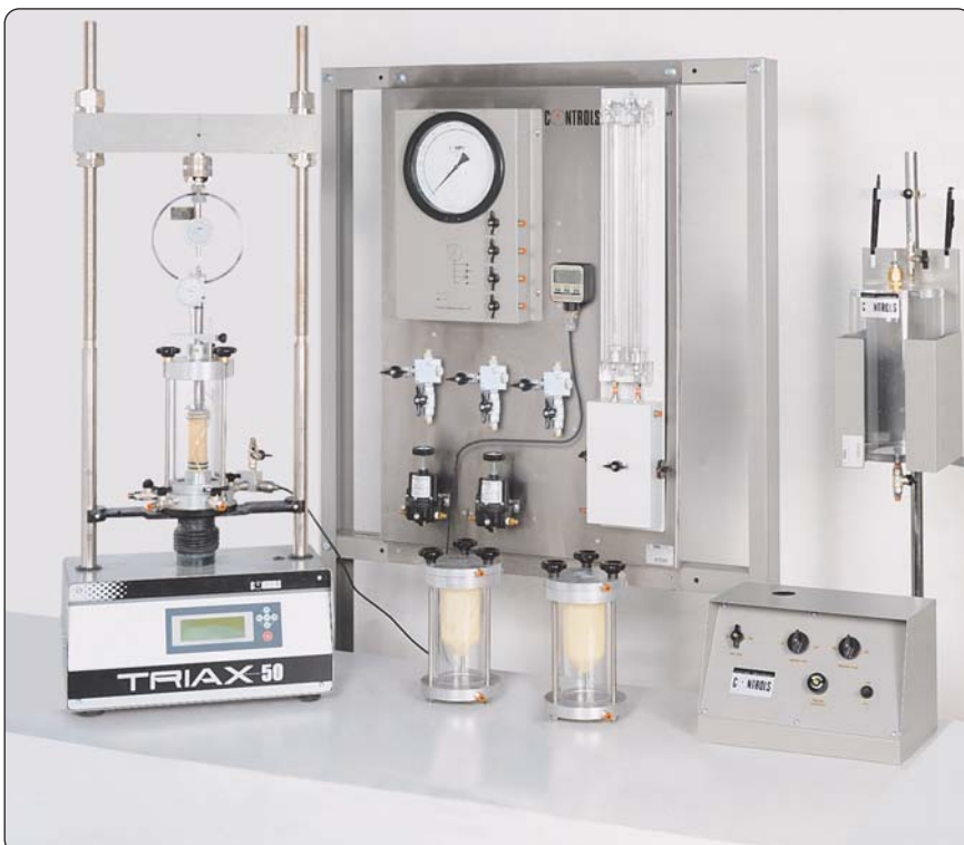
Pressure system for CU/CD test on one specimen with triaxial machine and cell
