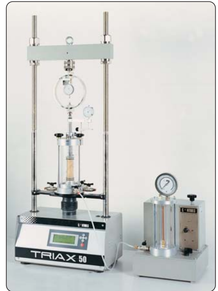
Pressure system 28-T0474/B with triaxial machine and cell
