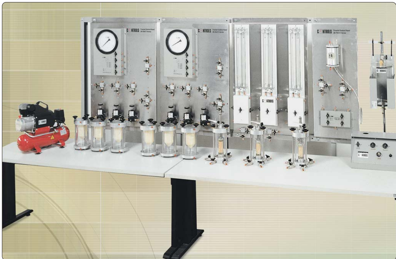
Typical pressure system for CU/CD tests on three cells (see layout on page 80)
