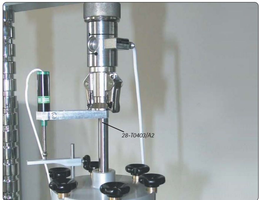
Detail of the triaxial cell and rigid connection to the piston for extension tests
