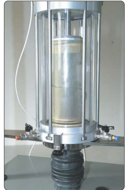
Detail of the locking system of the triaxial cell to the lower platen for extension tests
