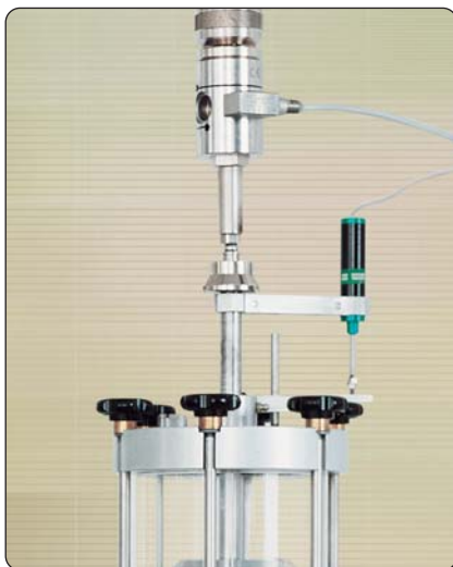
82-P0334 fitted to the triaxial cell by the 28-T1048 mounting bracket and 82-P0370/T load cell fitted to the frame by the spherical attachment
