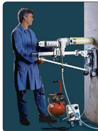
83-C0350 with vacuum attachment and vacuum pump during operation
