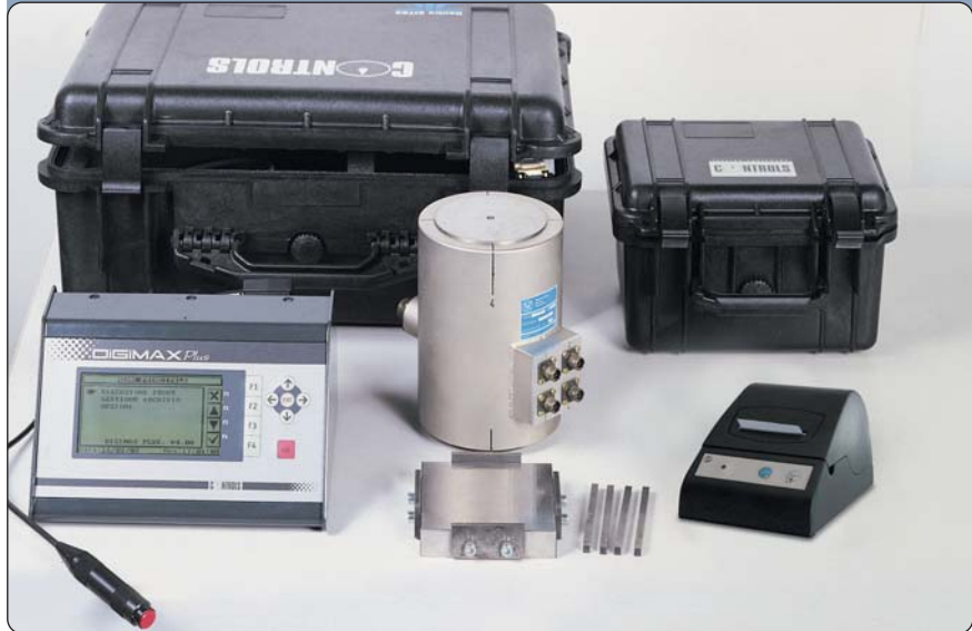
82-P0804/E with 82-E0105/1 Strain gauged column and 82-P0172 24-column printer that can be used to download the test results for further processing using programs developed by the user. The strain-gauged column is supplied complete with auxiliary platen and spacers for an easy and precise placing of the column either centrally or 6 mm displaced from the centre. It can be used as a 3000 kN load cell for force verification.
