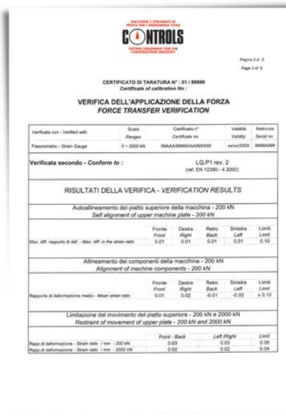
Final Force Transfer Verification certificate. The complete document includes other 3 certificates concerning upper plate self-alignment, alignment and restraint of movement.
