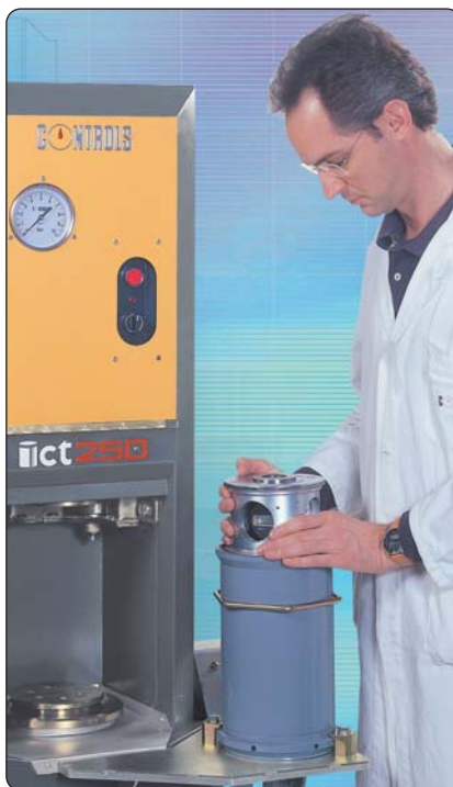
76-B0255 During calibration procedure. The ILS fits the 150 mm dia moulds without filling it with asphalt
