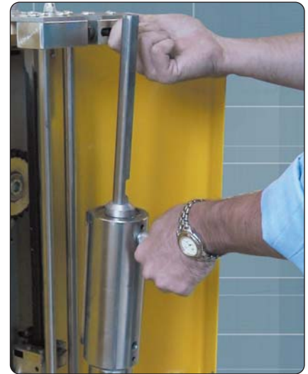
Detail of the rammer handling operation. The fast locking system allows easy maintenance operation, and the removable handle makes the rammer changing operation very fast and made by one person only
