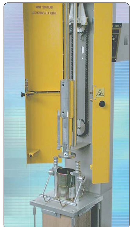
76-B4312 with open doors. When door is opened, the machine's automatically set in safety mode and cannot operate. In this conditions, all moving part are accessible for maintenance operations
