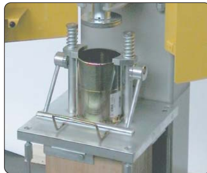
Detail of the mould clamping device. The new system, combined with the new mould, allows a really fast mould change operation in full operator safety condition
