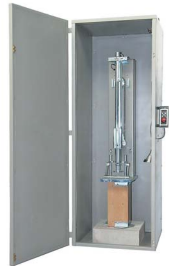
76-B4212 installed in the 76-B4200/XUP cubicle. Concrete base not included
