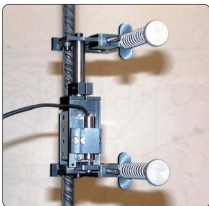
70-C0954/C Application on steel rebars
