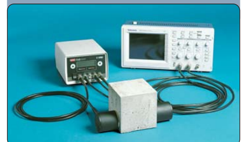
Ultrasonic tester 58-E0048 with oscilloscope 58-E0048/10
