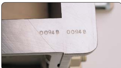
Detail of 55-C0101/A certified model (optional, add code 55-C0100/CAL). Each mould is verified and the serial number marked
