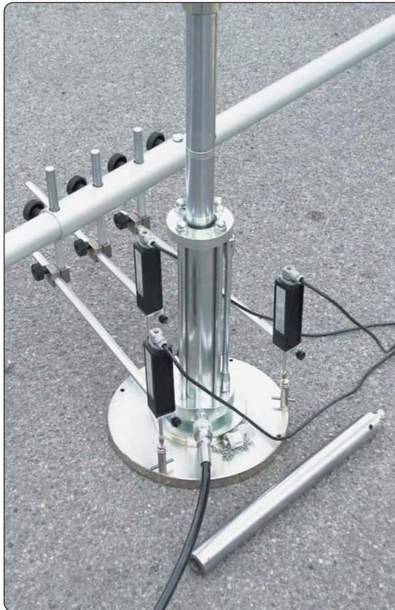
*Detail of the linear displacement transducers 50 mm travel with support and adjustable reference anvil*
