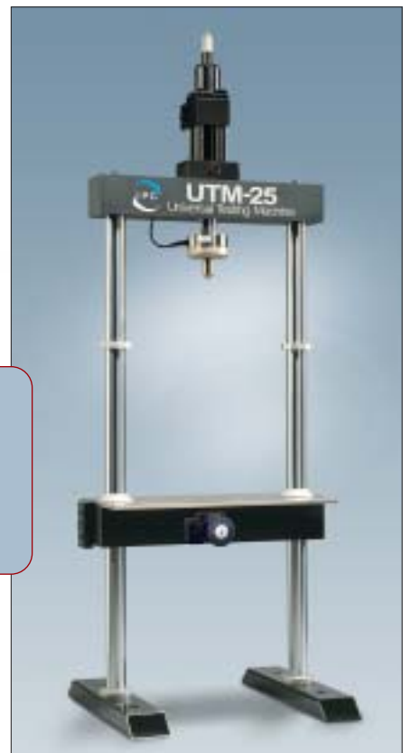
UTM-25 frame of the 77-B3202 servo-hydraulic system
