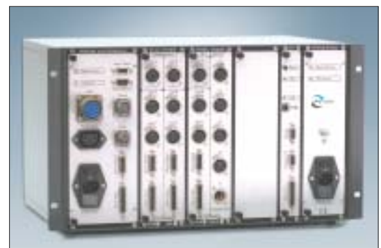
Detail of IMACS Control System, part of the load frames
