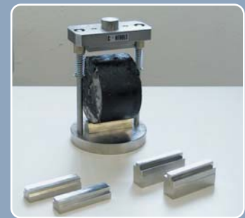
76-B0078/C tensile splitting device with 76-B0078/C1 and 76-B0078/C2 used to perform EN 12697-12 and EN 12697-23. See also page 352
